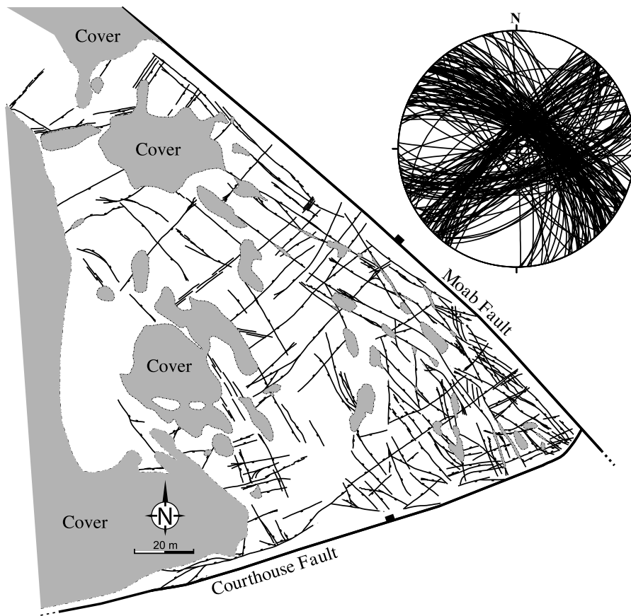
Figure 10. Map of deformation structures in the Courthouse branch point area and stereoplot (equal area, lower hemisphere) of the different structures in the same area. See Johansen et al. (in press) for a closer description.
